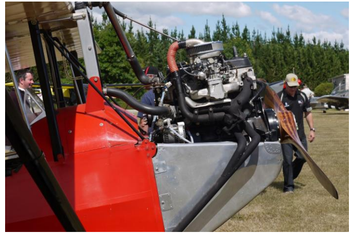
Evan and Penny Bellworthy's New Zealand Piet with Toyota Hilux 22R engine. About 100HP at 4800 RPM, perhaps 60HP without a redrive at speeds that won't get the propeller tips supersonic.
