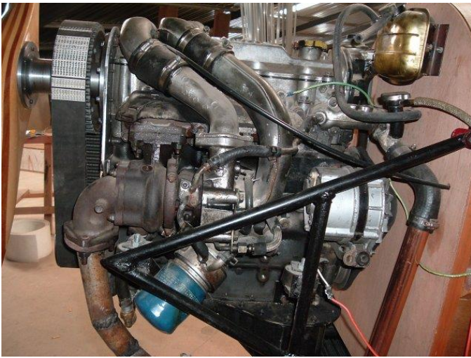
Toyota 2C turbo diesel on an Air Camper. About 87-90 HP without auto accessories.
